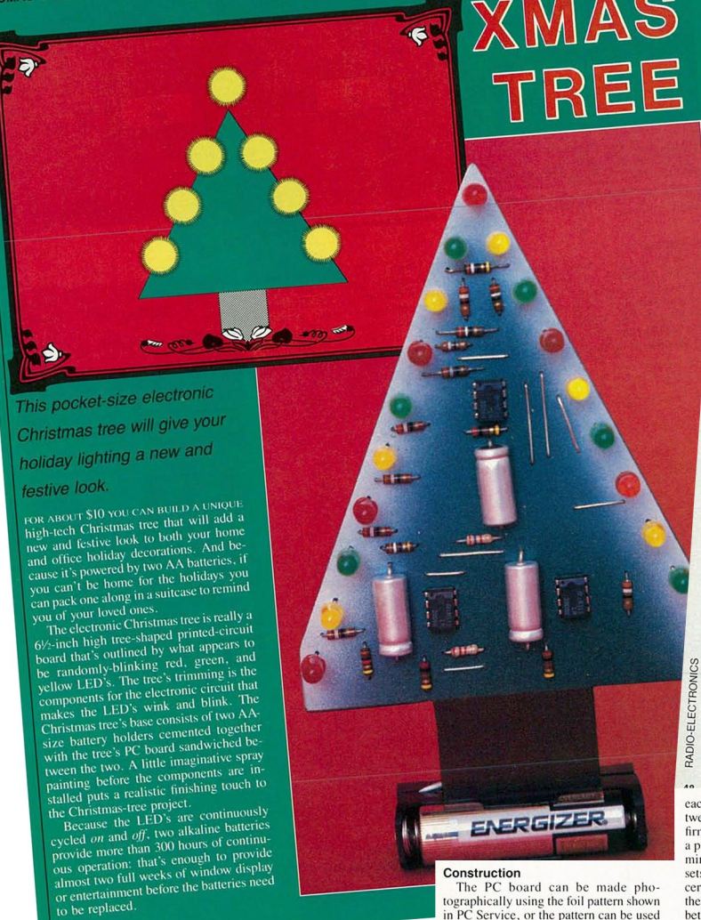
FIG. 1—THREE INDIVIDUAL FLASHER CIRCUITS having unrelated flash rates create a pseudo-random blinking of the LED's because the LED's from each individual circuit are intermixed around the edges of the tree.
